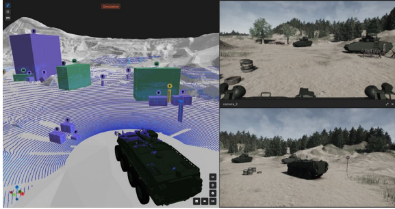
Figure 7 – Sensor Simulation in Applied Intuition’s Sensor Sim tool
