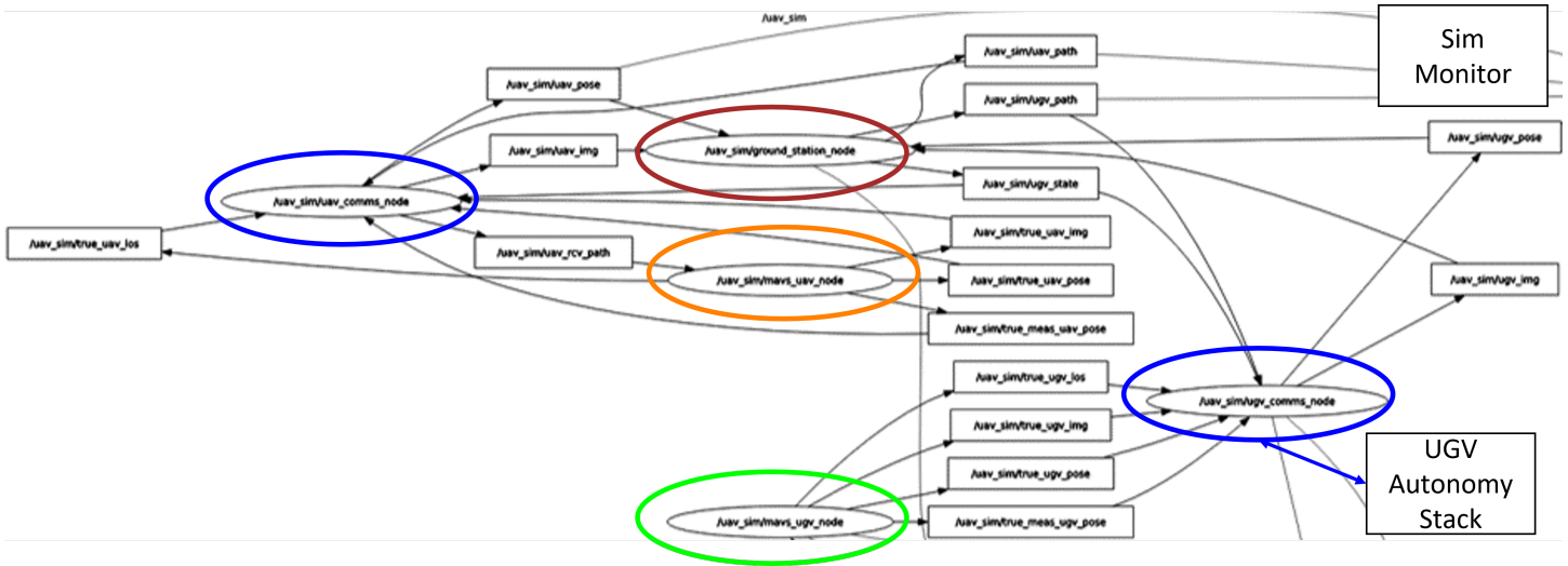
Figure 5: The ROS-2 network used to simulate the scenario shown in Figure 3
