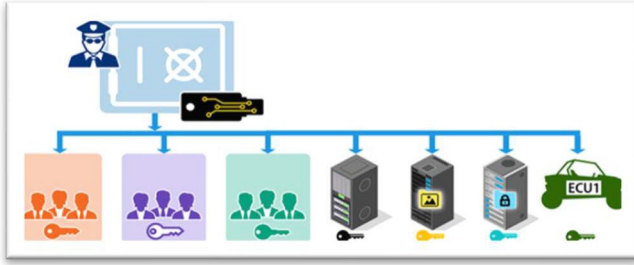
Figure 7. Different Roles in the Supply Chain use Keys to Approve Use of Software and Updates to the Security Policy. These Approvals are all Confirmed Prior to Installing Updates On-Vehicle
