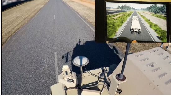
Figure 10: Virtual Leader Interacting with a Live Follower on a Digital Twin of ATC’s High Speed Test Track
