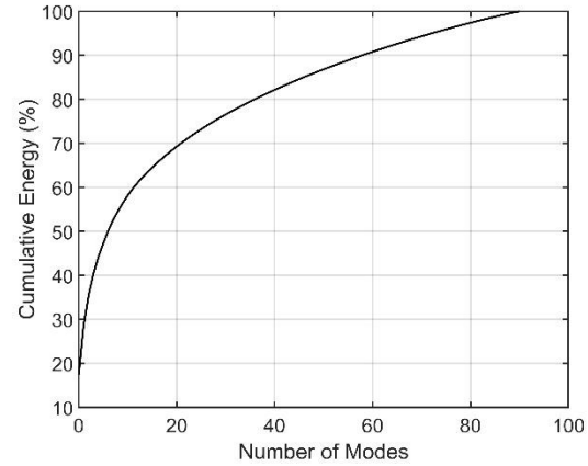
Figure 7: Cumulative energy of different modes from POD of the x-component of the velocity.
