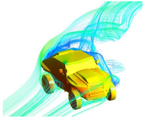
Figure 6: Visualization of flow over FED-Alpha for a wind angle of 55 degrees; streamline pattern showing separated region.
