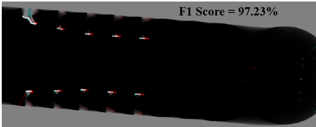
Figure 21: Comparison of Occupancy Maps. Black: Free in Both. White: Occupied in Both. Red: Higher Occupancy in Real LIDAR. Cyan: Higher Occupancy in Virtual LIDAR.
