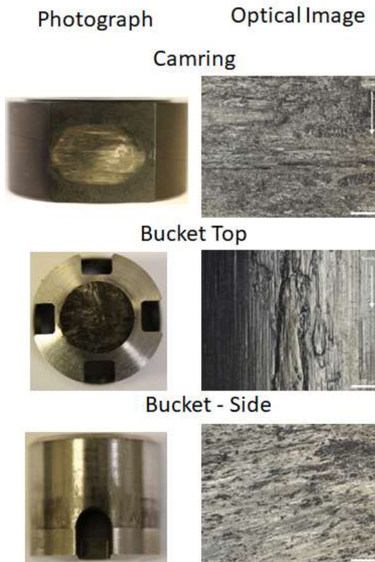
Figure 5: Photographs (left) and brightfield optical images (right) of damaged fuel pump sub-components from experiment with decane.
