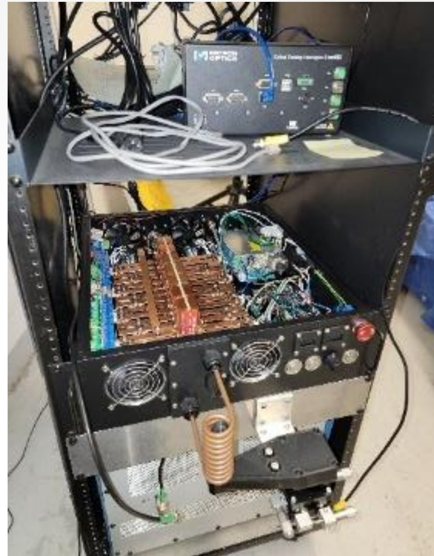
Setup for magnetic field excitation and melt-pool churning
