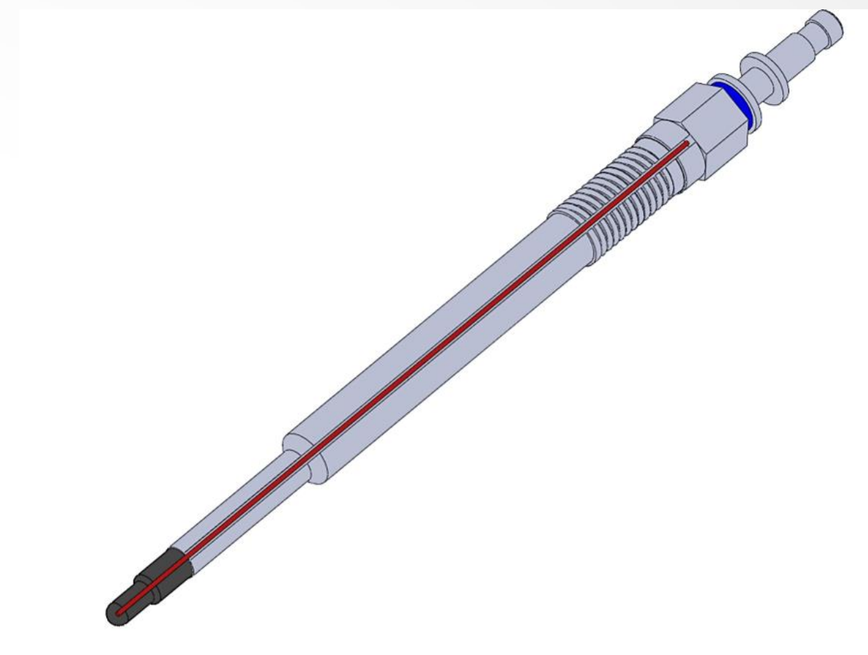
3D model of the modified ceramic glow plug used in the current work. The red line illustrates the path for the thermocouple installation
